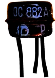
pnp-HF Germanium- transistor OC 882A
